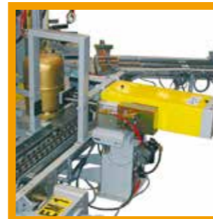
Tangential system Type: AT This device ensures automatic introduction of empty cylinders on the carousel filling scales. It is pneumatically driven and installed.
