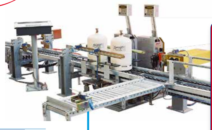
Electronic check scale Type: BCDA • Installed on chain conveyors • Production capacity : Up to 1,900 cylinders / hour
