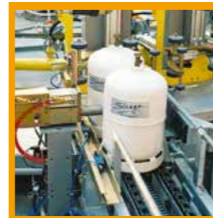
Pneumatic in-line admission with stop cylinder Type: AP This device ensures automatic introduction of empty cylinders on the carousel filling scales. It is pneumatically powered and installed at the end of the chain conveyor.
