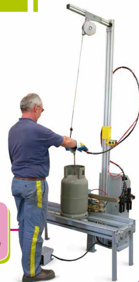
Removing residual unit Type: PADR • Residual water suction after inside washing or testing • Capacity up to 300 cylinders / hour • Manual version
