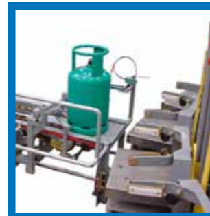
Pneumatic Radial in-line admission Type: AP This device ensures automatic introduction of empty cylinders on the carousel filling scales. It is pneumatically powered and installed at the end of the chain conveyor.
